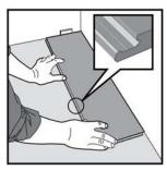
1. First plank, first row. Place a distance  $\frac{1}{4}$ " (5mm) thickness to the left and position the plank against the wall. Later, after 3 rows, you can easily position the flooring against the front wall with distances  $\frac{1}{4}$ ".
