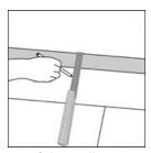
**10.** If the wall is uneven, the floorboards must be adapted to its contours. Mark the floorboards with the contour of the wall. Do not forget to leave a 1/4" space
