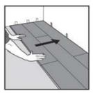
**9.** After 2-3 rows. Adjust the distance to the front wall by placing distances 1/4". Keep the distances in position during the entire time of installation and remove once the installation is completed.
