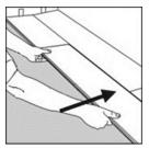
**8.** Push to slide the plank against the row in front so it aligns with the first plank. Put it down like with the first plank when the floorboards are positioned tightly together. The first/previous plank can now be folded completely down to horizontal position and if a wedge is used it can be moved to the next short end joint.
