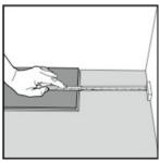
**3.** At the end of the first row, put a distance 1/4", to the wall and measure the length of the last plank to fit. Cut the last panel to correct length, recommended min length is two times the width of the plank.
