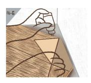
**16. Last row**Measure and cut the panels in the last row to size.
